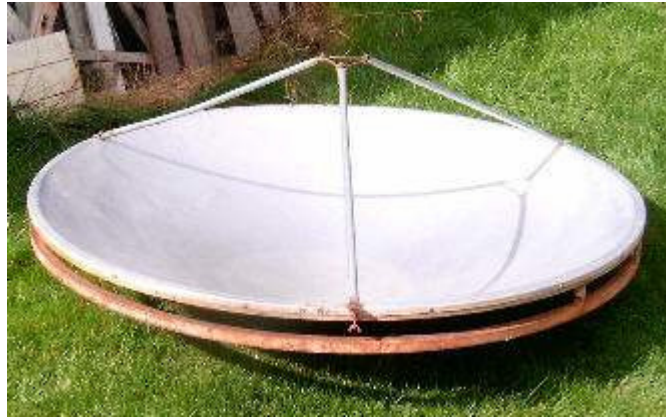
A 5 Foot Satellite Dish. This one is a 90 degree Focus Angle
